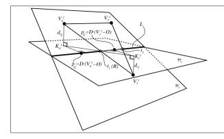
Figure 2: The geometrical situation:  $V_i^1$  are the vertices of  $T_1$ ,  $\pi_1$  &  $\pi_2$  are the planes in which  $T_1$  and  $T_2$  lie;  $d_{v_1}$  are the signed distances from  $V_i^1$  to  $\pi_2$ ;  $K_i^1$  are
